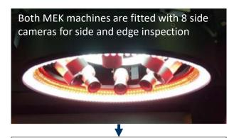
Combined with the central camera this provides a top down view for standard inspection and 8 side views.
