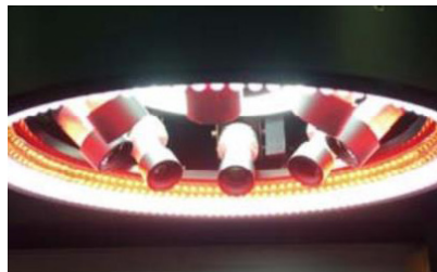
Both MEK machines are fitted with 8 sidecameras for side and edge inspection
