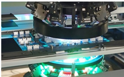
550 BTL with top & bottom cameras, for double sided inspection at the same time.
